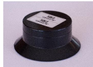
Figure 1: Long term radon detector
