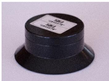
Figure 1: Long term radon detector
